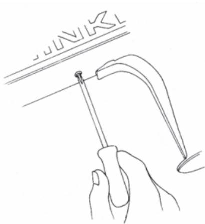
2.1 Undo screw (14) holding bracket (12).
