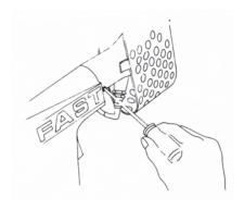
3.1 Undo spark plug clip (26A) undo screws (31) holding combustor and pull combustor off the body by twisting it.
