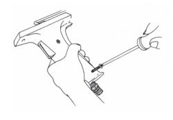
2.3 Remove front and rear screws (19) holding 2.4 handle. To reach the rear trigger (17A) must be depressed fully.
