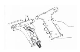
2.5 Separate handle halves for access to igniter fuel valve and triggers.
